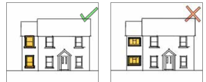
Figure 6: How to ensure that the pattern and detail of architectural features reflect those on the original dwelling
